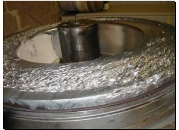
Figure 2 – Abrasion Caused by a Settling Slurry
